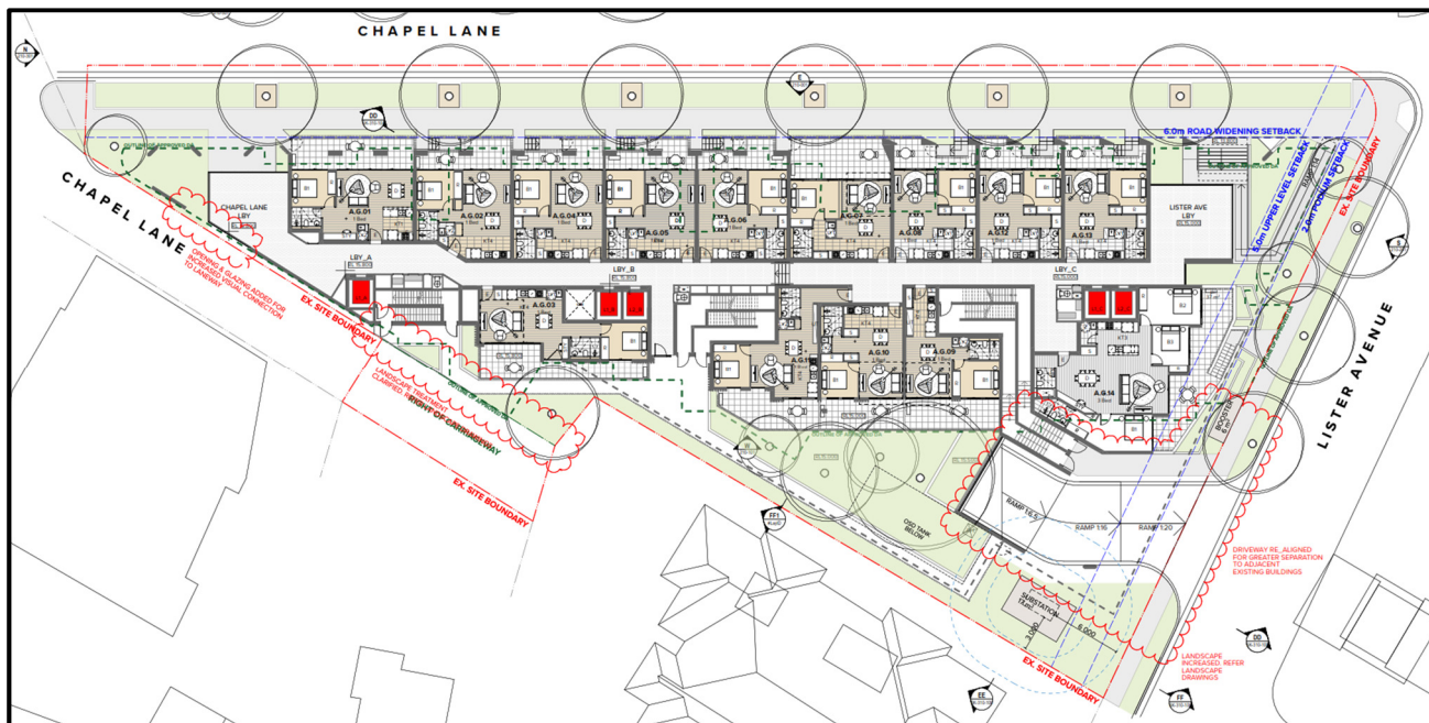
Figure 3: Extract from the proposed amended ground floor plan of Building A (Rev I)
